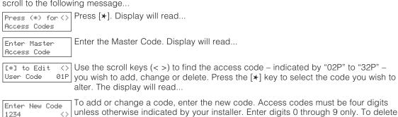
To add or change a code, enter the new code. Access codes must be four digits unless otherwise indicated by your installer. Enter digits 0 through 9 only. To delete an access code, enter [\*]. Once the 4 digit code or [\*] has been entered, the keypad sounder will beep 3 times and the display will read...
