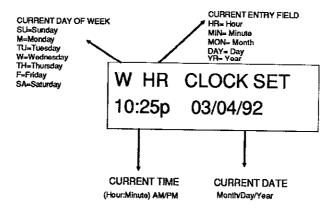
The top line shows the current time and the field being defined. The *INSTANT* key will be used to move between the fields and the *CODE* key is used to change between AM/PM.
