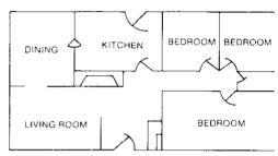
Smoke detector shall be located between the sleeping area and the rest of the house.
