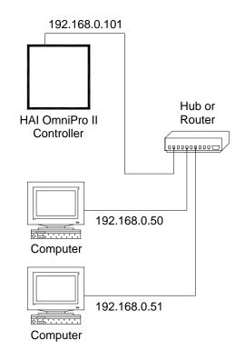
To connect to an OmniPro II controller on a local network using HAI PC Access, under *Configure* >> *Network* enter the controller's IP address:
